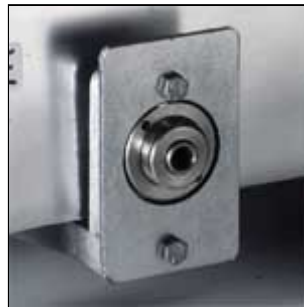
Device for releasing the carriage
